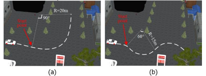
Fig. 8. Test scenarios. (a) a 90-degree bend with radius of curvature equal to 20m; (b) a S-Curve with radius of curvature equal to 15m. The white dash line is the designed track.
